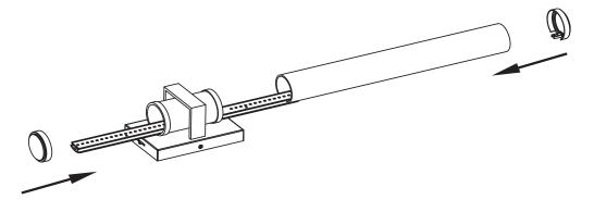
3. Install the glass holder with the 4PCS screws to secure the glass shade in place.
