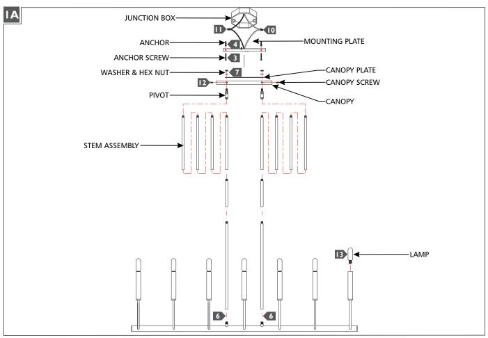
1 Temporarily install the mounting plate to the junction box.
