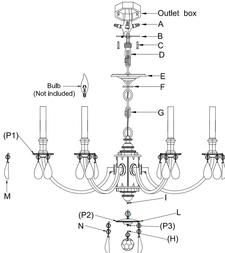
13. Attach the common wire (ribbed, no words) from the fixture to the white wire from the building using the provided wire nut(A).
