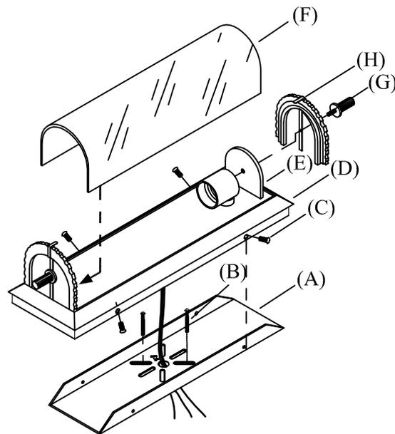
1. Attach ground (green) wire to ground wire from wall outlet box (usually green or copper in color), fasten together with a plastic wire connector. Tightly wrap the wire connector with electrical tape so the end of the connector is sealed. IT IS IMPERATIVE THAT THE OUTLET BOX IN YOUR HOME BE PROPERLY GROUNDED.
