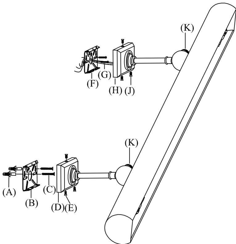
1. Remove back plates (B) and (F) from fixture bases (D) and (H) by unscrewing base screws (E) and (J).
