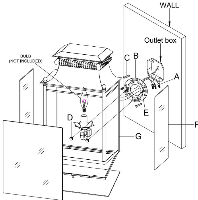
1. Remove the universal mounting plate from the outdoor lantern by removing the cap nuts.
