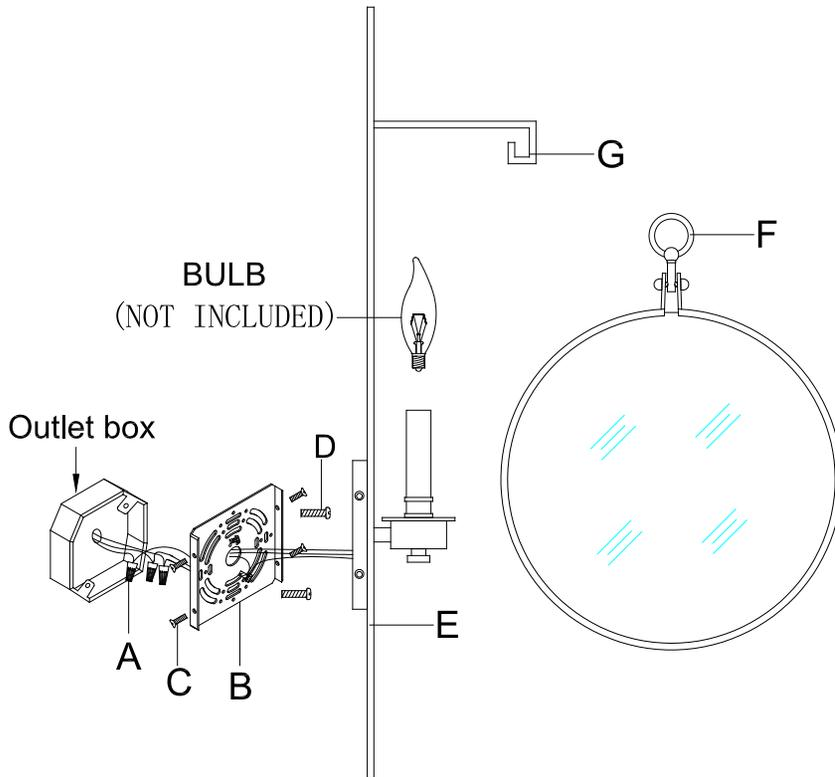
1. Carefully remove the mounting plate (B) from the back plate(E) by removing side screws(C).
