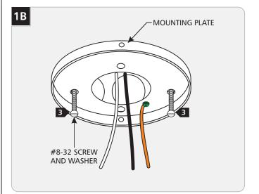
3 Secure the mounting plate to the electrical box with the two washers and #8-32 screws provided.
