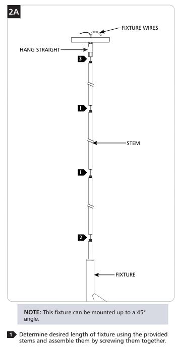
2 Feed the fixture wires through the stem assembly and screw it to the fixture.
