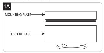
1 Unscrew the mounting plate from the fixture base.
