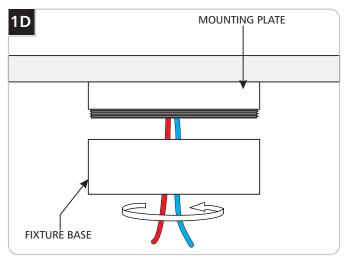
**7** Feed the transformer wires through the fixture base and tightly reinstall it onto the mounting plate.
