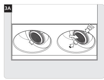
**WARNING:** Always squeeze the two tabs when adjusting the LED housing. Failure to do so will damage the finish.
