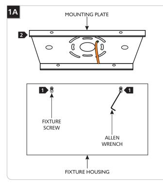
1 Remove the fixture screws located on both sides of the fixture housing using the provided Allen wrench.
