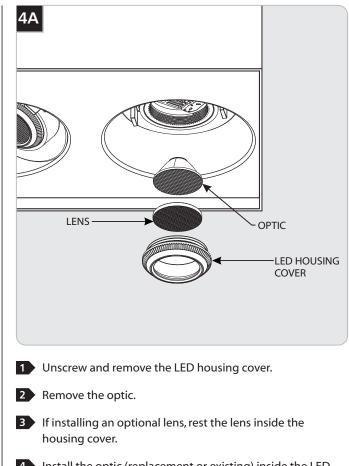
Install the optic (replacement or existing) inside the LED housing cover.
