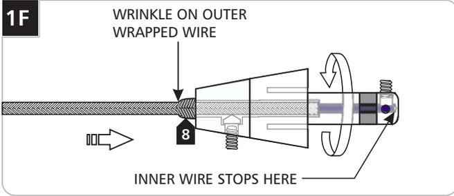
**8** Keep pushing the coaxial cable into the connector while rotating the connector to ease feeding the inner wire into the tip of the connector. The outer wrapped wire will start wrinkling while being inserted another 1/2" into the connector.
