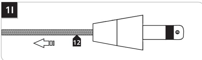
**12** Pull the coaxial cable toward the fixture to smooth the wrinkles.
