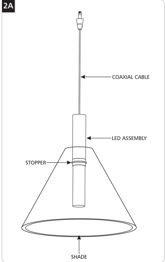
**1** Feed the coaxial cable through the shade and carefully lower the shade onto the stopper.
