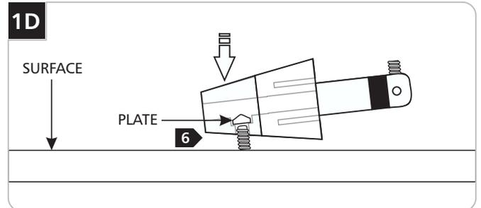
**6** Tap the conical connector on a hard surface with the set screw facing down, so the plate inside drops into place.
