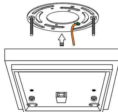
**3** Remove the mounting plate from the assembly by unscrewing the two knurled nuts.
