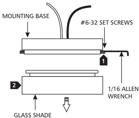
**1** While supporting the glass shade, loosen (**Do Not Remove**) the four #6-32 set screws on fixture base with the 1/16 Allen wrench.
