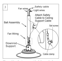
Thread lead wires provided through the long downrod and then Thread the safety cable provided through downrod (the end with loop installed downward) and connect it to the safety cable from fan (Parts are in the column). Slide cable clamp onto the safety cable from fan. Place the end of cable through the loop of ceiling support cable and then feed end of cable into clamp hole and firmly tighten set screw. Cut off excess safety cable and then pull the safety cable up from top of downrod.
