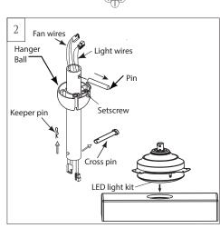
Remove hanger ball from existing downrod by loosening the set screw on hanger ball until the ball can be moved freely. Remove the pin and hanger ball from downrod. Keep the parts. Place fan assembly on styrofoam to keep the LED light kit away from damage and make fan installation easier. Flip the bottom styrofoam over, aligning
