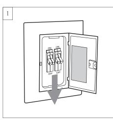
Before you begin handling parts replacement, Switch power off at Service panel and lock service disconnecting means to prevent power from being switched on accidentally. When the service disconnecting means cannot be locked, securely fasten a warning device, such as a tag, to the service panel.
