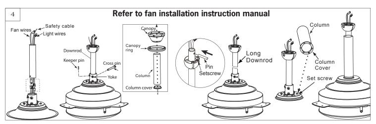
Note: Make sure to pull the safety cable up before you go next step of lead wires connection.
