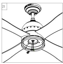
Isolate the quick connects with electrical tape.
