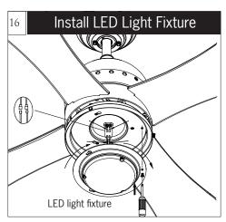
Connect white wire from fan to white wire from LED light fixture and then connect blue (or black) wire from light pan to black (or blue) wire from LED light fixture. Be sure plugs connection clasped together completely. Attach LED light fixture onto the light pan, aligning the keyhole slots on the LED light fixture with the preassembled screws on the light pan. Twist clockwise till lock. Reinstall the screw removed in the installation step 15. Tighten all screws securely.
