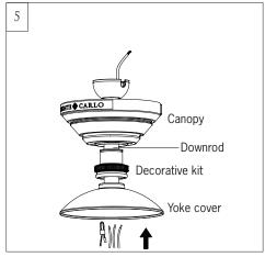
Place downrod over canopy, decorative kit and yoke cover. Thread lead wires and safety cable from motor assembly through downrod.
