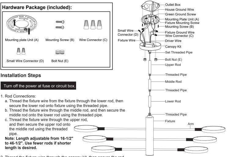
2. Thread the fixture wire through the canopy kit, then secure the rod assembly to the set threaded pipe of the canopy kit.
