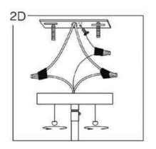
Lining up threads on mounting plate with holes in fixture canopy, attach fixture to junction box using cap nuts. Be sure to carefully tuck wires into canopy while attaching.
