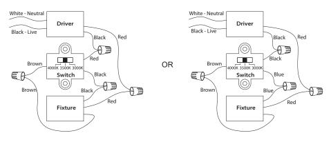
Note: Fixture will follow one of two wiring configurations shown. Identify which schematic is correct for your fixture by checking the switch wire colors.
