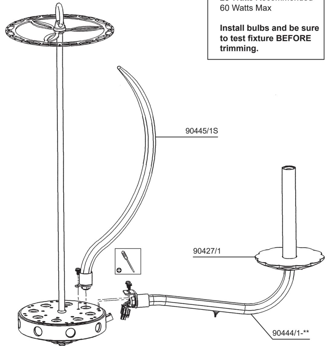
**19** Connect arm wires using plug-in connectors. See detailed illustration.
