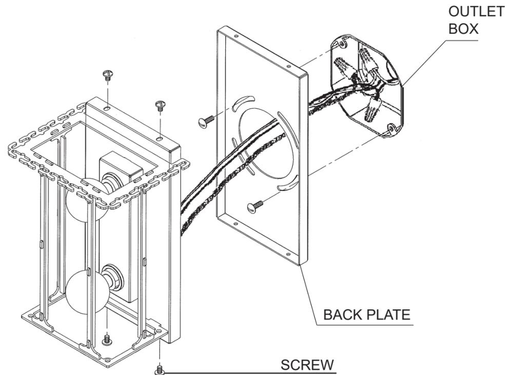
**3** Remove the (4) wall scone screws and separate the back plate from the wall scone. Feed stem and ground wires through back plate, then attach to power wires and ground wire in outlet box.
