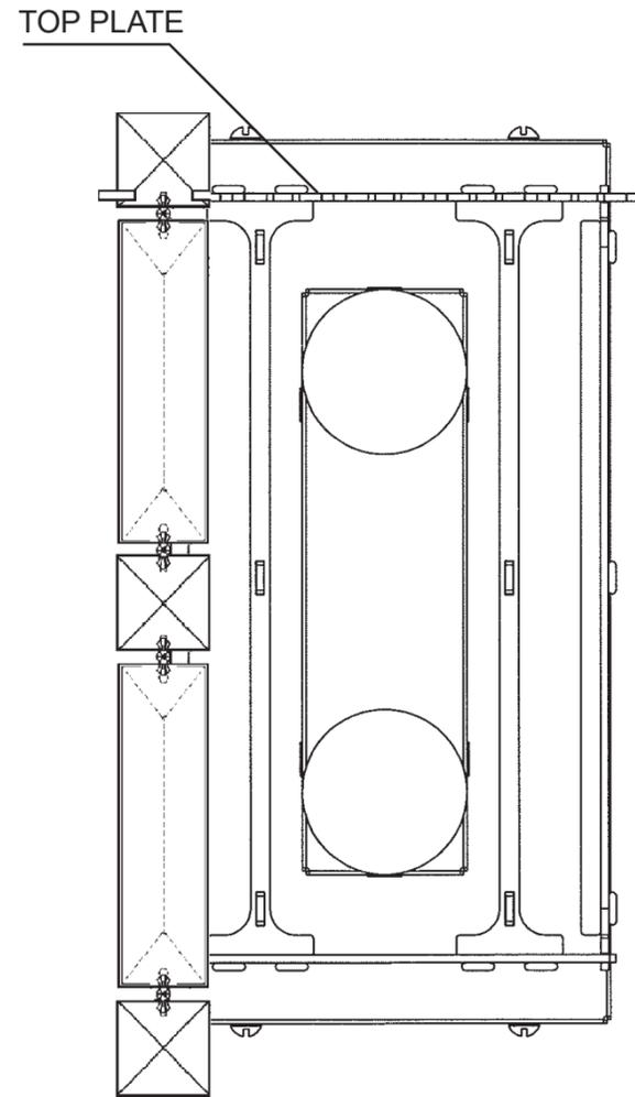
**7** Install bottom crystal grid with four thumb nuts (already screwed onto grid) to bottom of the wall sconce.
