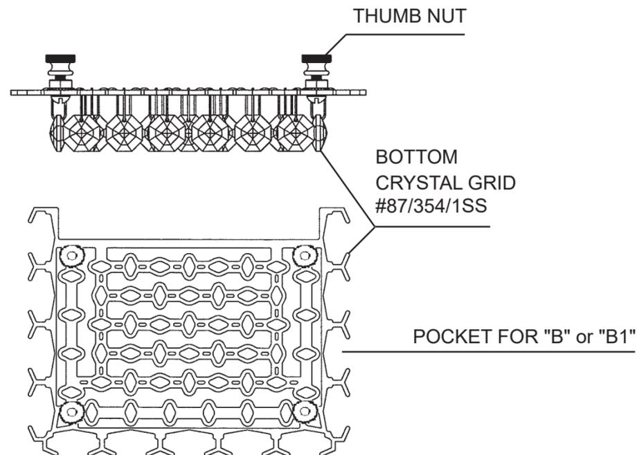
**7** Install bottom crystal grid with four thumb nuts (already screwed onto grid) to bottom of the wall sconce.
