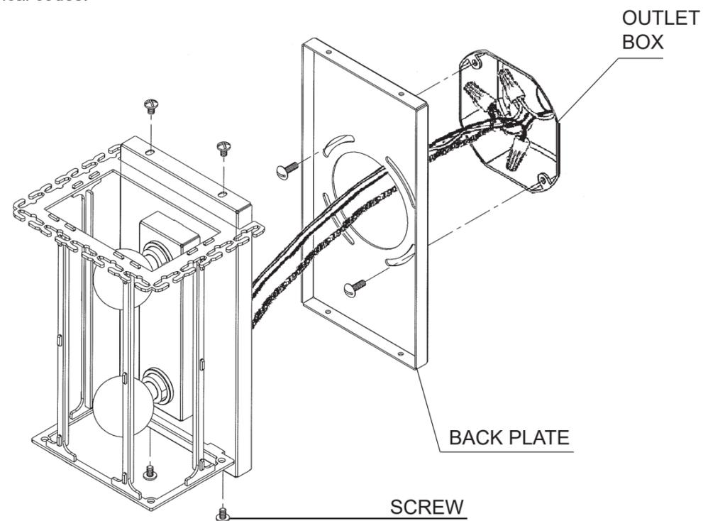
**3** Remove the (4) wall sconce screws and separate the back plate from the wall sconce. Feed stem and ground wires through back plate, then attach to power wires and ground wire in outlet box.
