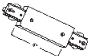
To connect two track sections together in a straight line. Add 4" to length, can be used as a power feed.
