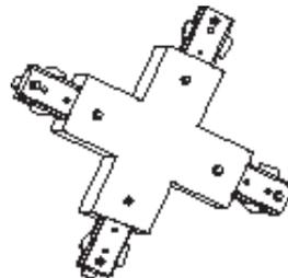
To connect four track sections in a X configuration. Can be used as a power feed. Add 4" to length.
