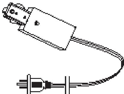
Live end feed with cord and 3-prong plug. 10-Amp 12-foot ground cord.
