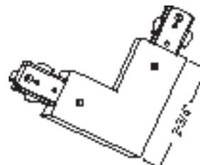
To connect two track sections at a 90° angle. Field adjustable for right or left polarity. Can be used as a power feed. Add 2-3/4" to length.
