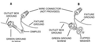
Make wire connections (connectors not provided). Reference chart below for correct connections and wire accordingly.
