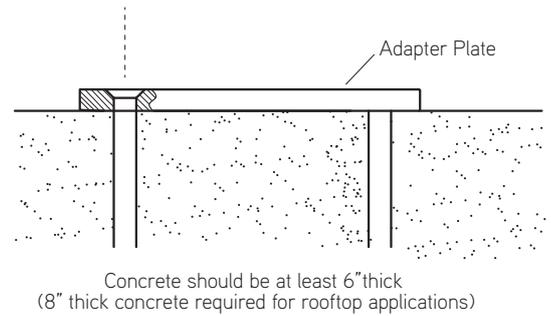
**3** Insert (4) expansion bolts into countersunk holes and tighten using an allen wrench.
