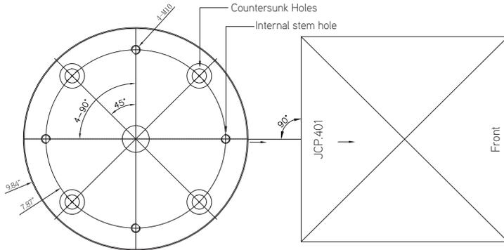
**2** Make sure all adapter plate holes align with drilled holes in concrete.
