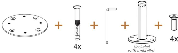
**1** To achieve the exact desired position of the JCP401, it is imperative that the adapter plate and internal stem be aligned correctly. One of the 4 internal stem holes must face direction of umbrella. Drill (4) holes on concrete according to countersunk holes in diagram below. Hole depth should be no less than 4" / 100mm.
