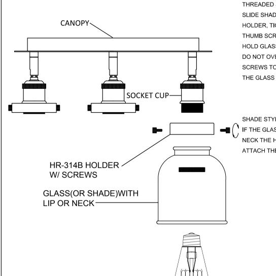
**BALLSTON URBAN ASSEMBLY** ATTACH THE HR-314B HOLDER TO THREADED SOCKET CUP USING THREADED SOCKET RING SLIDE SHADE INTO THE HR-314B HOLDER, TIGHTEN THE (3) THUMB SCREWS EVENLY TO **HOLD GLASS IN PLACE** DO NOT OVER TIGHTEN THUMB SCREWS TO AVOID BREAKING
