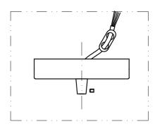
PASSING THE WIRE THROUGH THE CANOPY SECURED TIGHT WITH SET SCREW, THEN PUT THE WIRE CLIP ON THE WIRE END TO HOLD THE WIRE.
