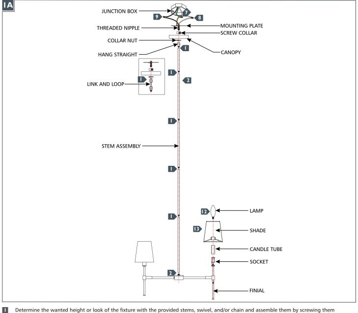
together. NOTE: Use hang straight for standard ceilings and use link and loop for sloped ceilings.
