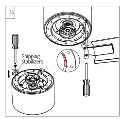
Remove shipping stabilizers from motor assembly.
