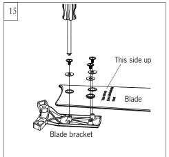
Install blade onto blade bracket with provided set screws and washers. Tighten screws securely. Repeat this process for remaining blades.
