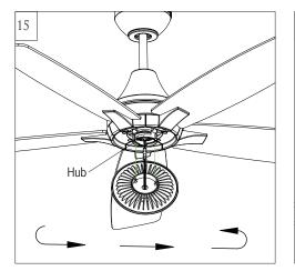
Install the LED light fixture onto the hub on the fan.
