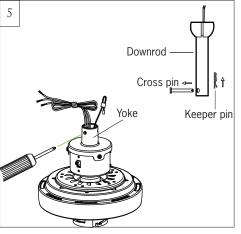
Partially loosen downrod set screws from yoke at top of motor assembly. Remove preassembled keeper pin and cross pin from downrod. Keep parts
