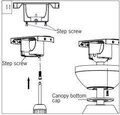
Partially loosen one and remove one preassembled step screw from mounting bracket (Do not remove the other set screws). Save the screw. Lift canopy up, aligning its keyhole slot with the preassembled step screw on mounting bracket and twist clockwise to lock in place. Reinstall the other step screw and tighten the screws securely. Attach canopy bottom cap onto canopy by aligning its holes with the step screws on mounting bracket and fix it with the magnet embraced.
