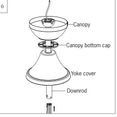
Place downrod over canopy, canopy bottom cap and yoke cover. Thread lead wires and safety cable from motor assembly through downrod.
