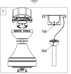
Install ball end of downrod into mounting bracket opening. Align (engage) slot on ball with tab on mounting bracket. **Warning:** Failure to align slot on ball with tab may result in serious injury. **Important**: If using the angle mount, make sure open end of mounting bracket is installed facing the higher point of the ceiling and make sure the ceiling angle is not steeper than 20°. Longer downrod may be necessary allowing the fan blades to rotate without obstructions.
