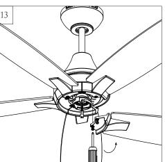
Install the blade assembly to motor using the preinstalled screws. Tighten screws securely. Repeat this process for remaining blade assemblies.
