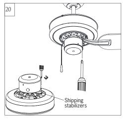
Remove shipping stabilizers from motor assembly.
