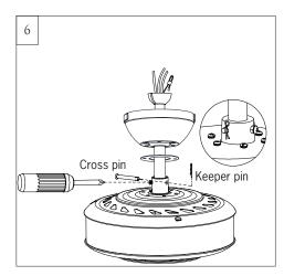
Slip downrod into motor housing yoke, aligning holes and install cross pin and keeper pin.
