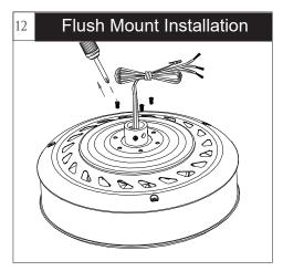
Remove every other screws from yoke located on top of fan assembly. Keep screws.
