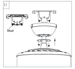
Lift Canopy allowing the 2 studs to protrude through the canopy.
