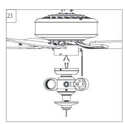
Connect light lead wires. White to white, blue (or black) to black (or blue). Make sure the quick connectors are clasped firmly.
