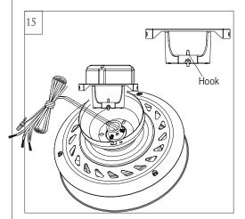
To prepare the fan for wiring, hang fan onto mounting bracket by sliding the canopy over the mounting bracket hook (Use one of non-slotted holes on the rim of the canopy).
