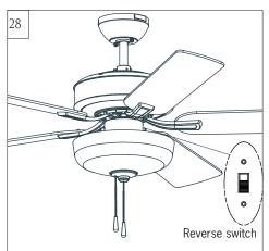
Setting the reverse switch in the down position will result in downward airflow and setting the switch in the up position will result in upward airflow.
