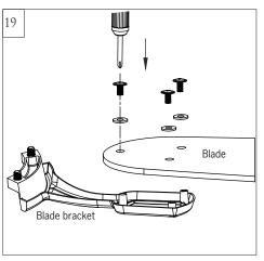
Install blade bracket with blade by 3 blade screws and washers provided. Tighten screws securely. Repeat this process for remaining blades.
