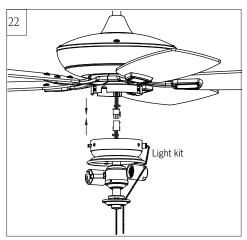
Connect the plug from fan with the plug from light kit. Be sure plugs connection clasped together completely.
