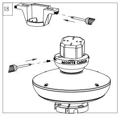
Install 2 of the screws to the side panel of mounting bracket corresponding to the open slotted holes on the canopy upper rim, screws provided. Remove the all thread studs from the lower part of the mounting bracket.
