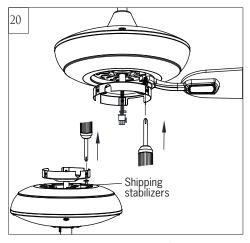
Remove shipping stabilizers from motor assembly.
