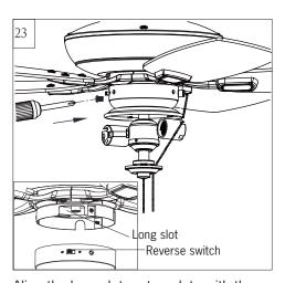
Align the long slot on top plate with the reverse switch on light kit, and then install the light kit onto the top plate with the 3 set screws removed in step 21 and tighten all screws securely.
