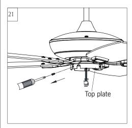
Remove the 3 set screws on top plate of light fixture, keep screws.
