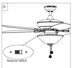
Setting the reverse switch in the left hand side will result in downward airflow and setting the switch in the right hand side will result in upward airflow.
