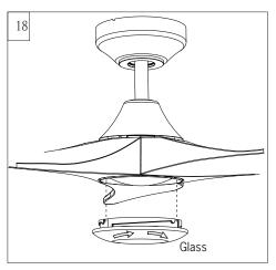
Attach glass by locating dimples in light pan with grooves on the glass and twist clockwise until tight.
