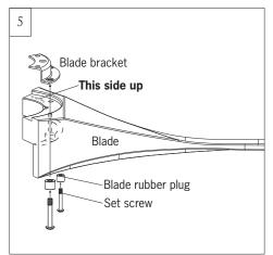
Note: Make sure the side with a label "This side up" is installed upward. Aligning the holes on blade and the screw holes on blade bracket as shown in illustration, and then partially install the set screws with blade rubber plug. Screws provided. Tighten screws securely after 2 set screws are installed. Repeat this process for remaining blades. Caution: Make sure the blade rubber plug is in position.
