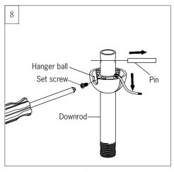
Remove hanger ball from downrod by loosing the set screw and removing the pin as shown in illustration. Keep parts.
