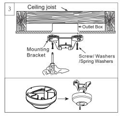
Partially loosen one screw corresponding to the round hole on the canopy and remove the other preassembled screw from mounting bracket. Save screw. Remove the canopy from the mounting bracket.
