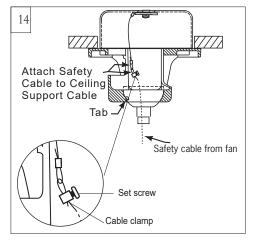
Connect the safety cable from fan to the Ceiling support cable.
