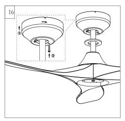
Lift canopy up, aligning its keyhole slot with the preassembled screw on mounting bracket and twist clockwise to lock in place. Reinstall the screw removed in step 3 and tighten all screws securely. Do not over tighten it.
