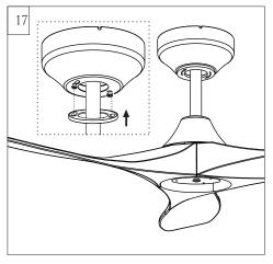
Attach canopy bottom cap onto canopy by aligning its notch with the screws on mounting bracket and twist clockwise till tight.
