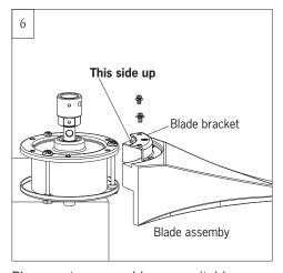
Place motor assembly on a suitable area of paper pulp for installation of blade assembly.
