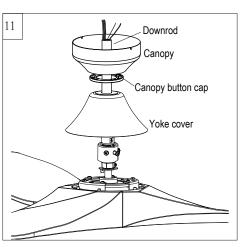
Place yoke cover, canopy bottom cap and canopy over lead wires, safety cable and downrod.
