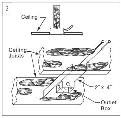
Before installing this fan makes sure the outlet box is properly installed to the house structure. Ensure the outlet box is securely fastened by at least two points to a structural ceiling member (a loose box will cause the fan to wobble). To reduce the risk of fire, electric shock, or personal injury, mount to outlet box or supporting system acceptable for fan support.
