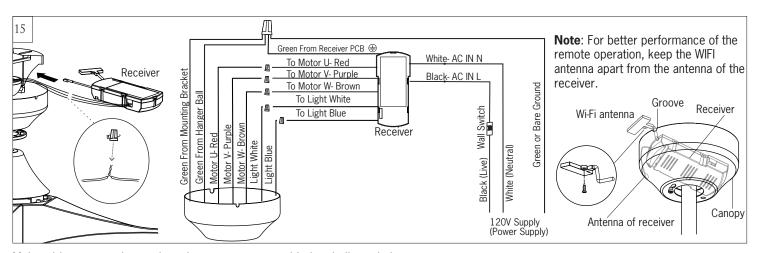
Make wiring connections using wire connectors provided as indicated above.
