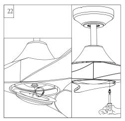
Attach LED light fixture onto the light pan, aligning the keyhole slots on the LED light fixture with the preassembled screws on the light pan. Twist clockwise till lock. Reinstall the screw removed in step 20. Tighten all screws securely.
