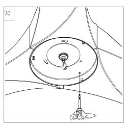
Loosen 2 and remove 1 preassembled screw from light pan. Save screw for later use.
