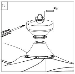
Replace the hanger ball with pin and set screw. Tighten it securely. **Warning**: Make sure the **pin** is installed well on hanger ball with downrod.
