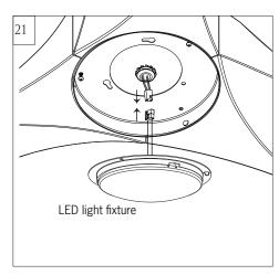
Connect light lead wires from fan to the lead wires from LED light fixture with quick connectors. Make sure the quick connectors are firmly clasped.
