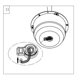
Connect the lead wires from fan to the quick connector on light fixture. Make sure the quick connectors are clasped firmly.
