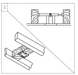
Before installing this fan make sure the outlet box is properly installed to the house structure. To reduce the risk of fire, electric shock, or personal injury, mount to outlet box or supporting system acceptable for fan support. (Mounting must support at least 35 lbs.) Use metal outlet box suitable for fan support and use only the screws provided with the outlet box (must support 35 lbs). Before attaching fan to outlet box, ensure the outlet box is securely fastened
