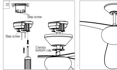
Partially loosen one and remove one preassembled step screw from mounting bracket (Do not remove the other set screws). Save the screw.
