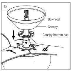
Place canopy bottom cap and canopy over lead wires, safety cable and downrod.
