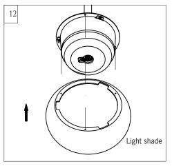
Attach the light shade onto the light fixture.
