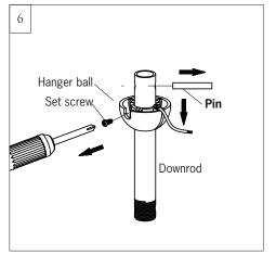
Remove hanger ball from downrod by loosing the set screw and removing the pin as shown in illustration. Keep parts.
