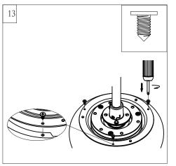
Corresponding to the last installation step and fix the light shade by the self tapping screws provided. Do not overtighten.
