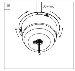
Attach the light fixture onto the adapter on the motor. Align the raised dimples in the light fixture with the grooves on the adapter as shown in the illustration and turn it clockwise till tight.
