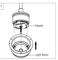
Remove the **black** cable tie from the light lead wires. Feed the light lead wire over the central hole at bottom of the light fixture.
