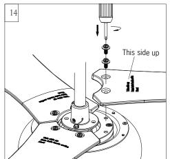
Place the motor assembly on a suitable area of paper pulp for blade installation. Install a blade onto the motor with set screws provided. Repeat this process for the remaining blades. Tighten all the set screws securely.
