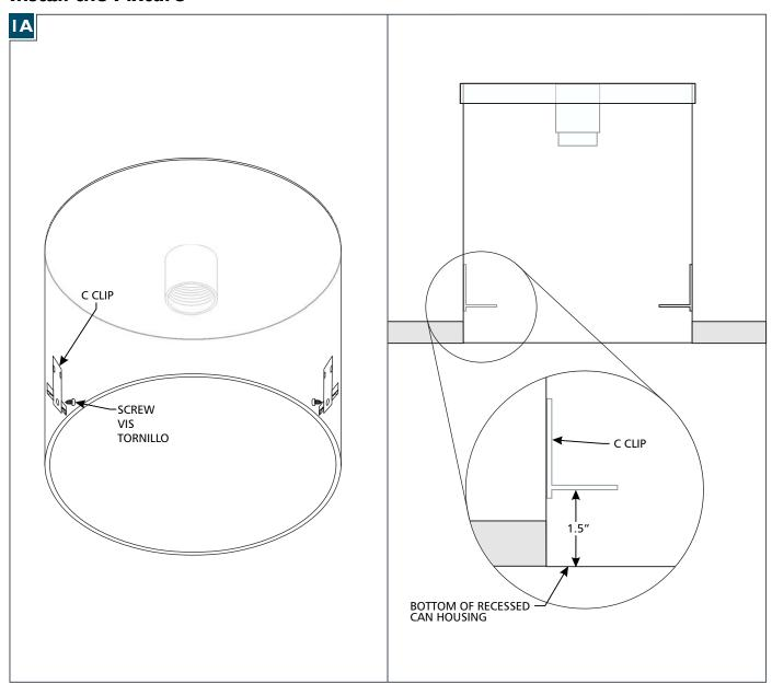
Using the provided self-tapping screw, install the c clip approximately 1.5" from the bottom of each side of the recessed can housing. Ensure that the c clips are leveled and directly across from each other.
