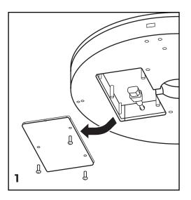
Remove the wiring compartment cover.
