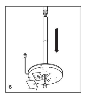
Feed the LED and power cables through the middle pole, bottom pole, and base of the unit. Screw the top pole into the middle pole.
