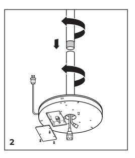
Thread the bottom pole into the base. Next, thread the middle pole into the bottom pole.
