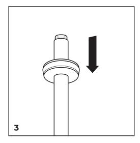
Insert the LED diffuser through the top pole.
