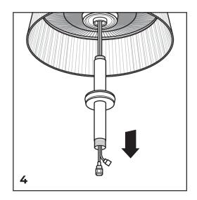
Feed the power cords from the unit assembly through the top pole.
