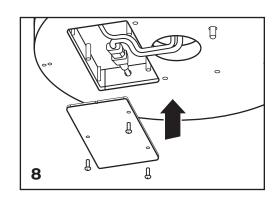
Reinstall the wiring compartment cover.
