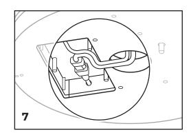
Connect the LED and power cables in the base of the unit.
