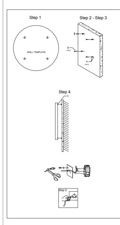
1.) Place the wall template of the mirror on the wall in the location selected for the mirror. Make sure the wall template or mirror is level and in the correct position. Secure the wall template to the wall then mark location of the 4 wall anchors(A) as indicated on the template from the wall. Remove the wall template from the wall.
