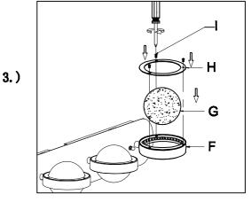
Step.3: Place bubble glass sphere (F) into cup and secure using ring (G).
