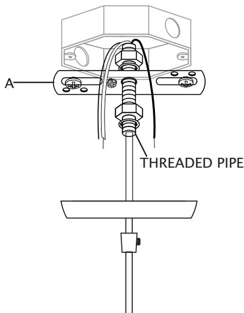
10. Slightly loosen ground screw on mounting bracket (A). Do not completely remove ground screw. Wrap house ground wire (copper) around ground screw, leaving enough ground wire to attach to fixture ground wire. Twist end of fixture ground wire and end of house ground wire (copper) together. Twist wire connector (C) onto ends of wires. Completely tighten wire connector (C). Reference chart below for correct wire connections.
