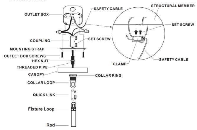
NOTE:NEC CODE (314.24) requires that ceiling outlet boxes in the United States support up to 50 lbs. This fixture exceeds 50 lbs. and must be installed using an outlet box approved for up to 100 lbs. or independently of the existing outlet box. Installation hardware and instructions are provided for both.
