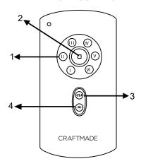
Fan **SPEED** buttons--1: Use to control ceiling fan speeds 1-6 Fan **OFF** button--2: Use to turn the fan off
