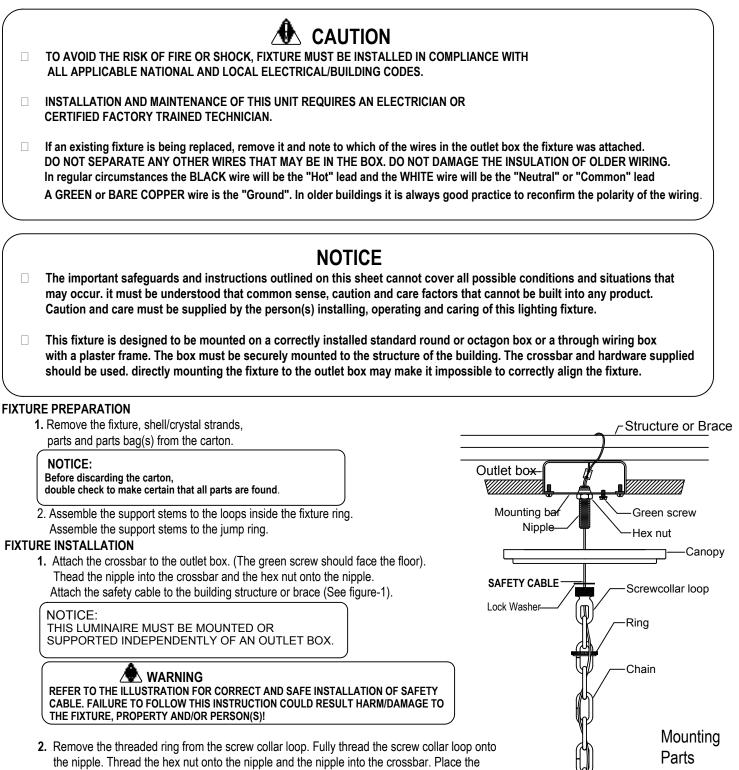
the nipple. Thread the hex nut onto the nipple and the nipple into the crossbar. Place the canopy over the screw collar and against the ceiling. Adjust the nipple so that 1#4" of threads on the screw collar loop extend beyond the canopy. Tighten the hex nut against the crossbar. Using the threaded ring, install the canopy.
