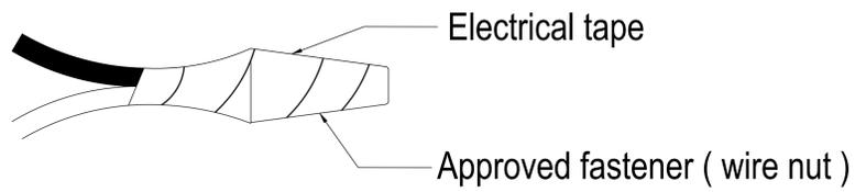
3. Connect the black fixture lead to the black wire in the outlet box. Fasten the joined wires as in step 3.
