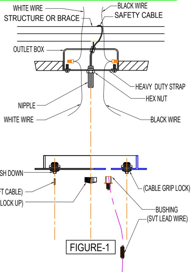
5. Attach the heavy duty strap to the outlet box using the mounting screws. Attach the safety cable to the building structure or brace.(Refer Figure-1).
