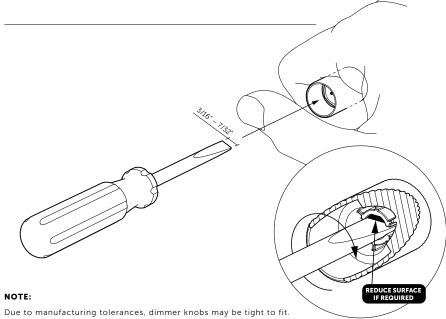
To allow for easier assembly, insert a  $3/16^{\circ} - 7/32^{\circ}$  (5 – 5.5mm) flat head screwdriver and rotate 360° to remove excess material from the flat section of the insert.
