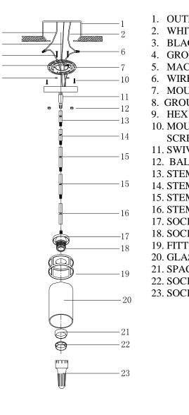
1. OUTLET BOX 2. WHITE WIRE 3. BLACK WIRE 4. GROUND WIRE 5. MACHINE SCREW 6. WIRE CONNECTOR 7. MOUNTING BAR 8. GROUND SCREW 9. HEX NUT 10. MOUNTING **SCREW** 11. SWIVEL 12. BALL NUT 13. STEM 14. STEM **15. STEM 16. STEM 17. SOCKET CUP** 18. SOCKET **19. FITTER** 20. GLASS 21. SPACER 22. SOCKET RING 23. SOCKET WRENCH
