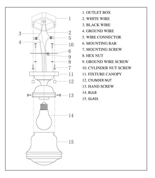
Line art shown may not exactly match the fixture enclosed. However, the installations do apply to this fixture. ITEM NO: 735F10 736F10
