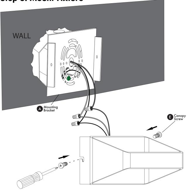
Attach fixture to mounting bracket (A). Secure with canopy screws (E). Tighten with Phillips head screwdriver.
