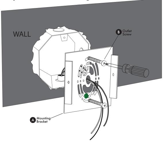
Align mounting bracket (A) with outlet box and secure with outlet screws (B).
