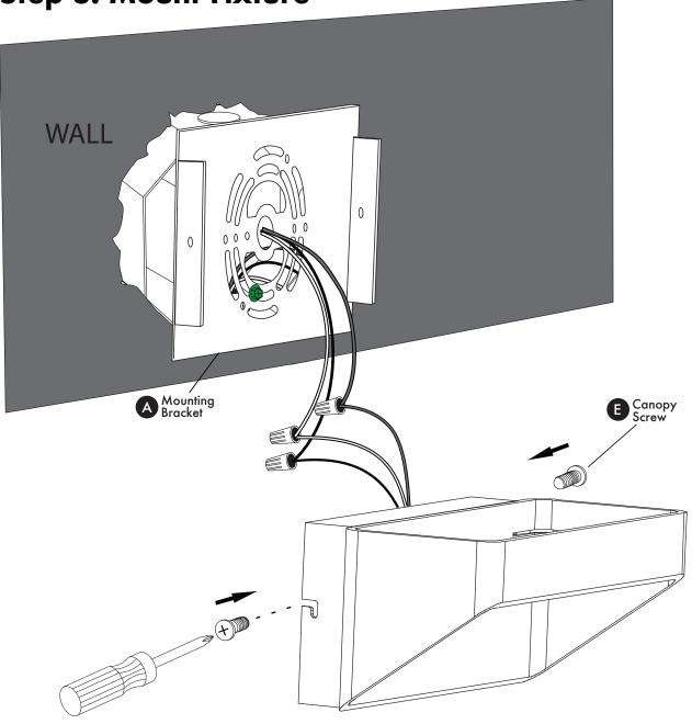
Attach fixture to mounting bracket (A). Secure with canopy screws (E). Tighten with Phillips head screwdriver.
