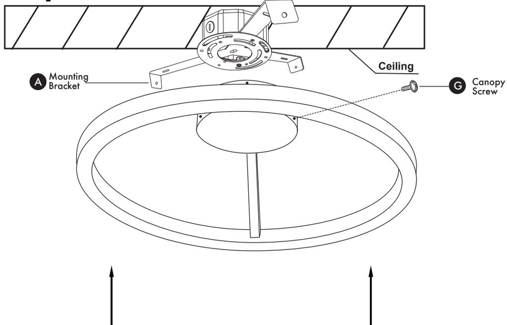
Attach fixture to mounting bracket (A).
