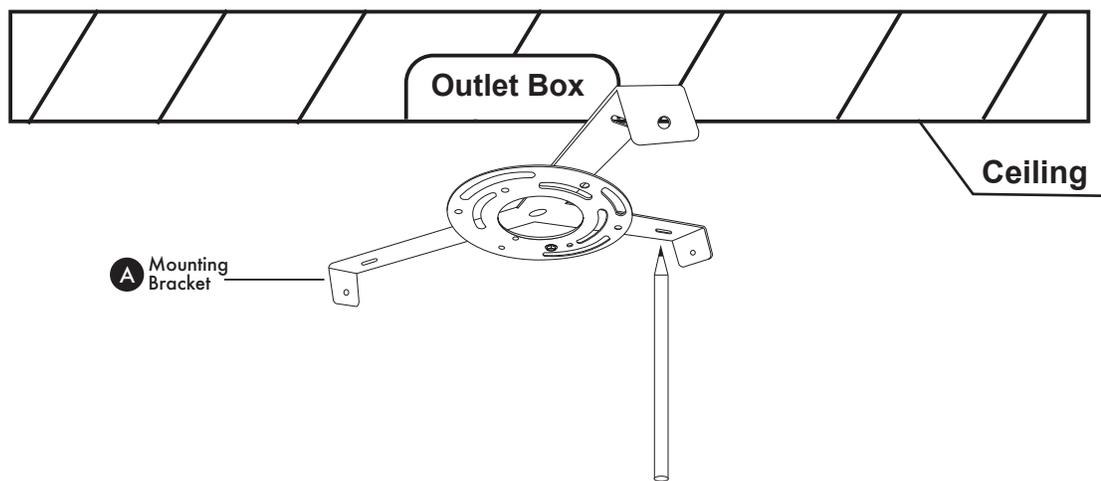
Remove mounting bracket (A) from fixture. Raise mounting bracket (A) to the ceiling. Mark location for the plastic anchors (B). Drill holes for plastic anchors (B). Insert plastic anchors (B) into hole.
