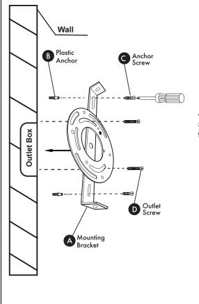
Raise mounting bracket (A) to the wall. Mark location for the plastic anchors (B). Drill holes for plastic anchors (B). Insert plastic anchors (B) into hole.
