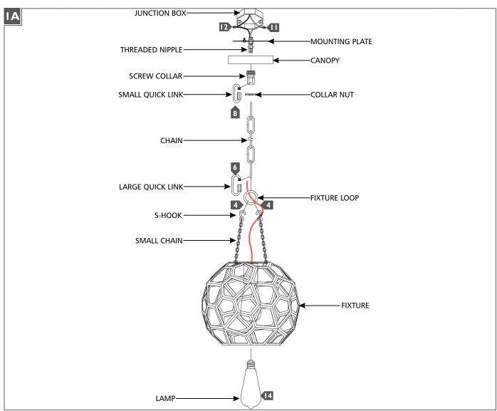
If necessary, screw the short end of the threaded nipple tightly onto the mounting plate.
