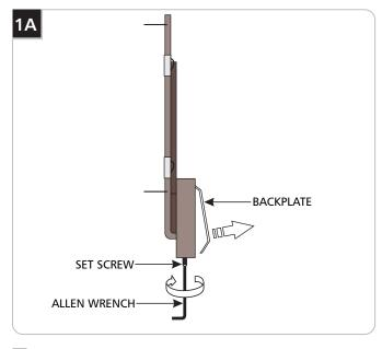
Loosen (do not remove) the set screw at the bottom of the fixture and remove the backplate.
